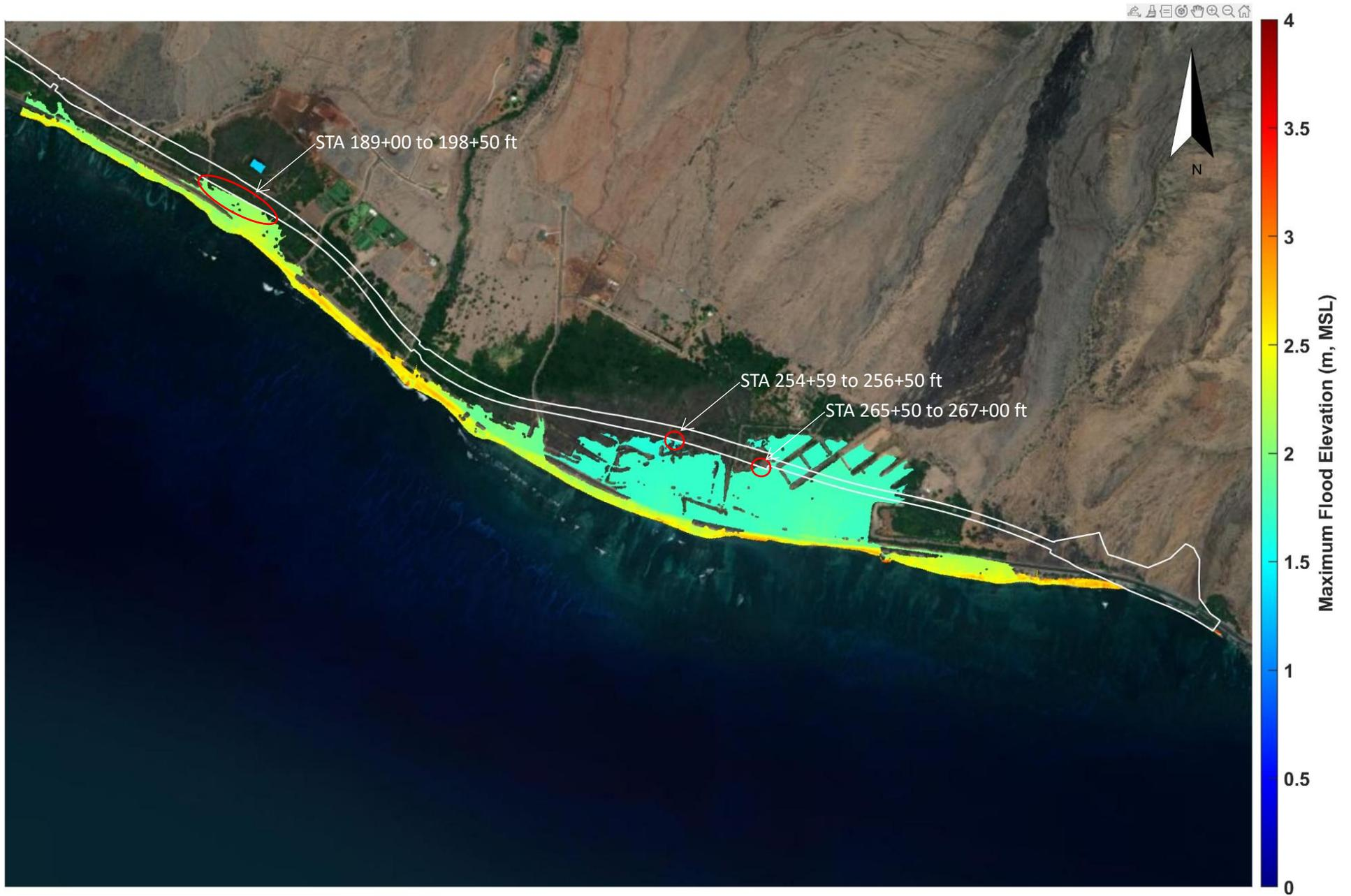
Figure C-2. XBeach-NH modeled maximum flood elevation for alternative 1 alignment (Ukumehame)
