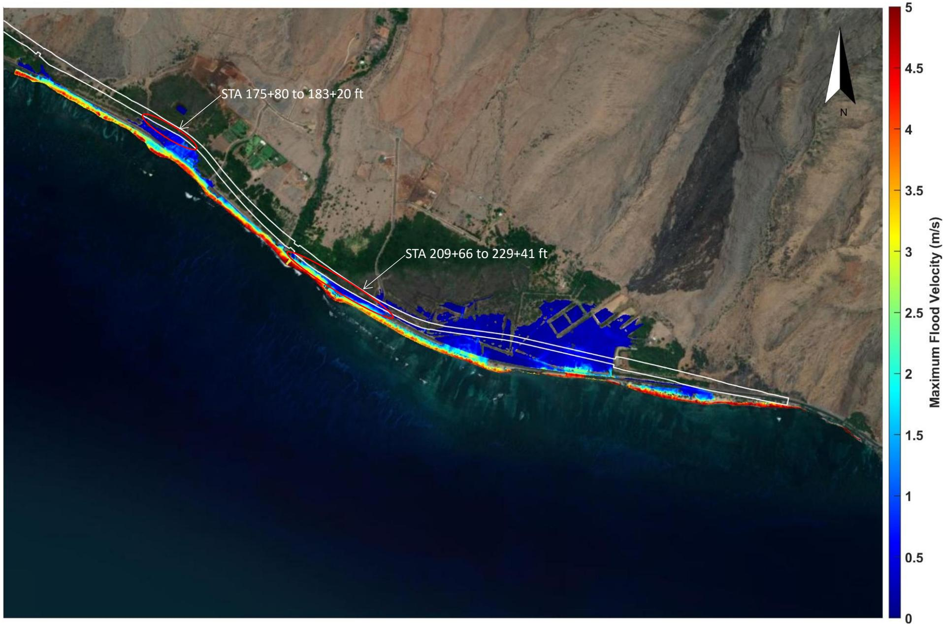
Figure E-3. XBeach-NH modeled maximum flood depth-averaged velocity for alternative 3 alignment (Ukumehame)
