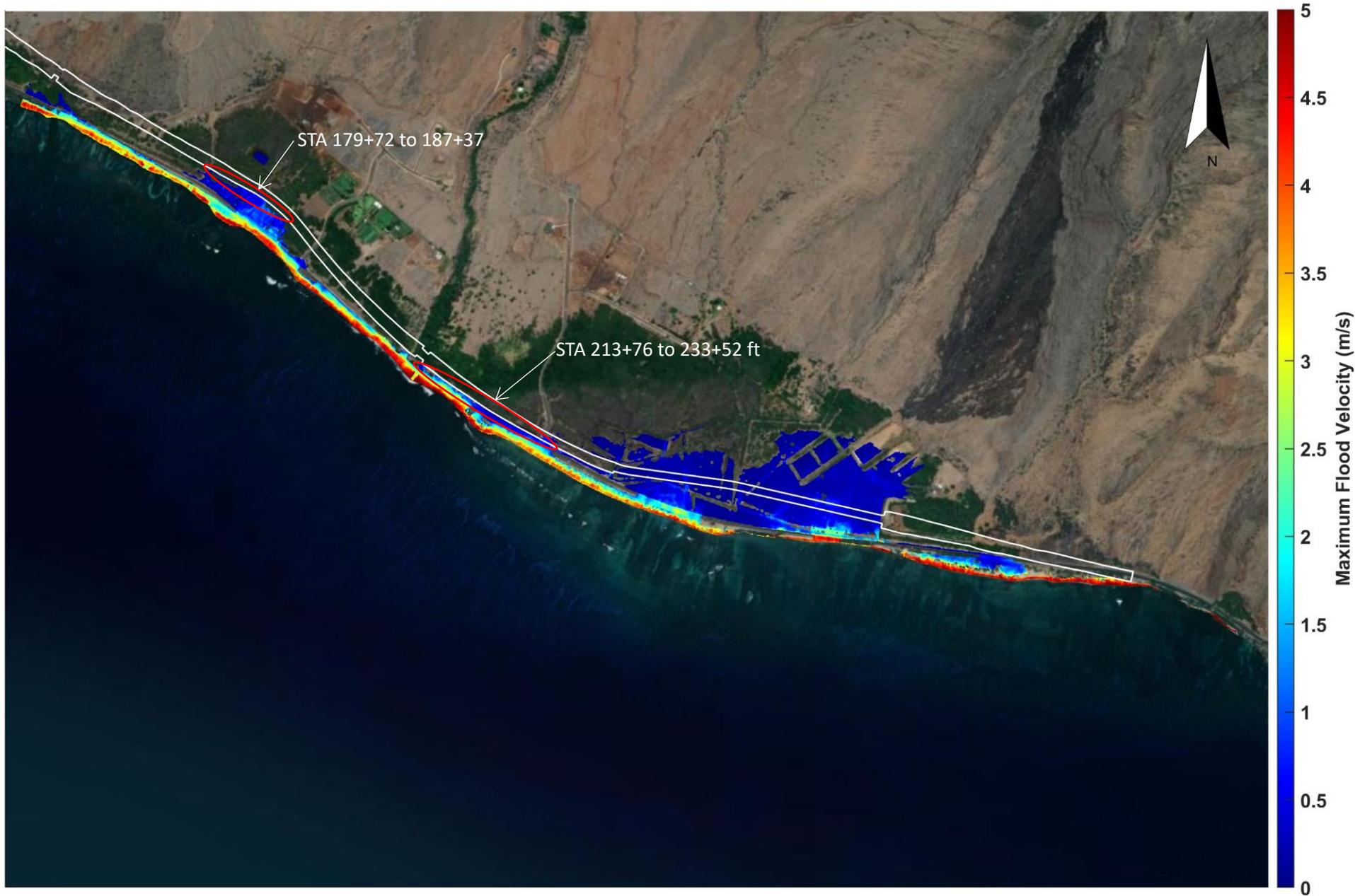
Figure D-3. XBeach-NH modeled maximum flood depth-averaged velocity for alternative 2 alignment (Ukumehame)
