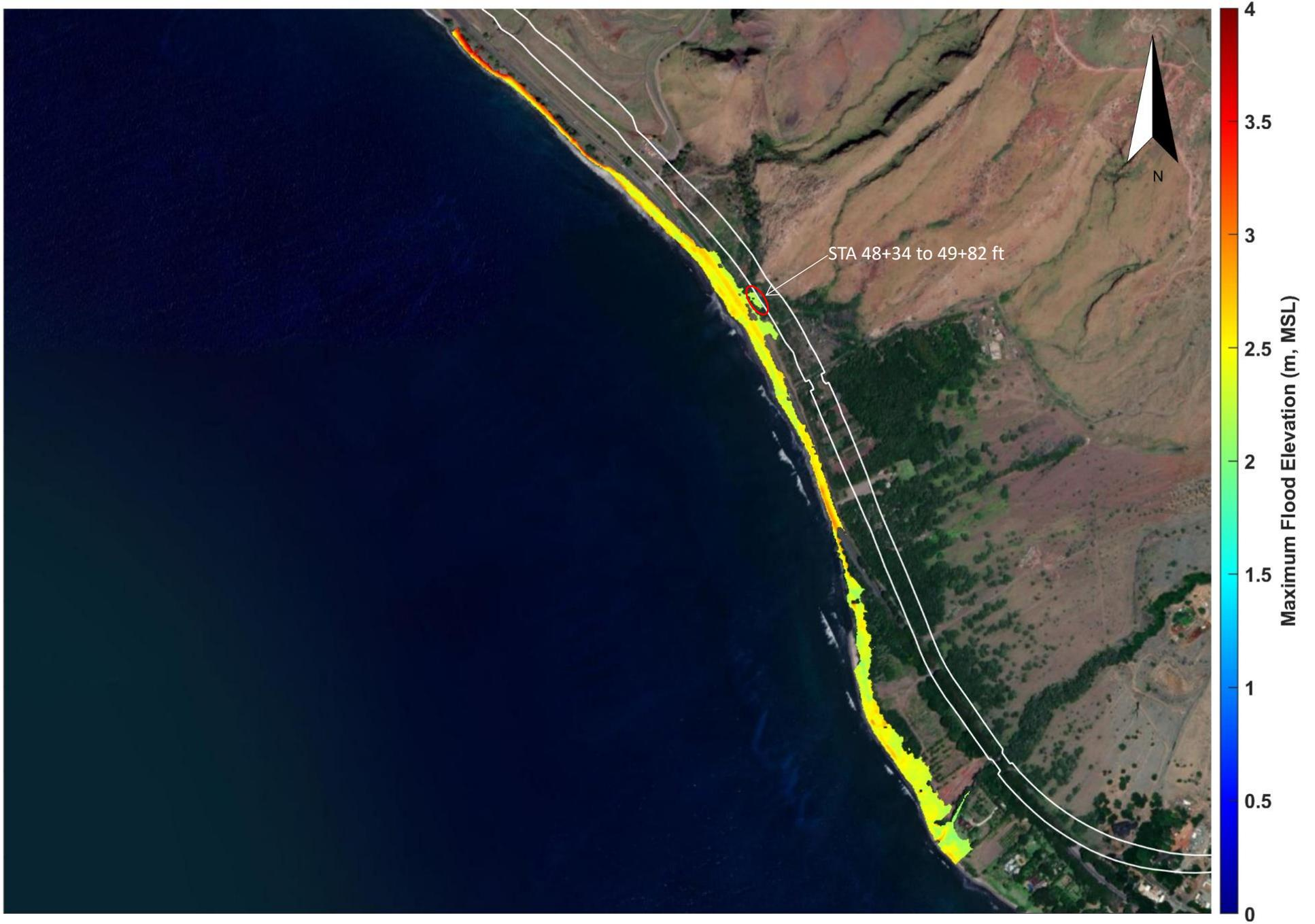
Figure C-5. XBeach-NH modeled maximum flood elevation for alternative 1 alignment (Olowalu)
