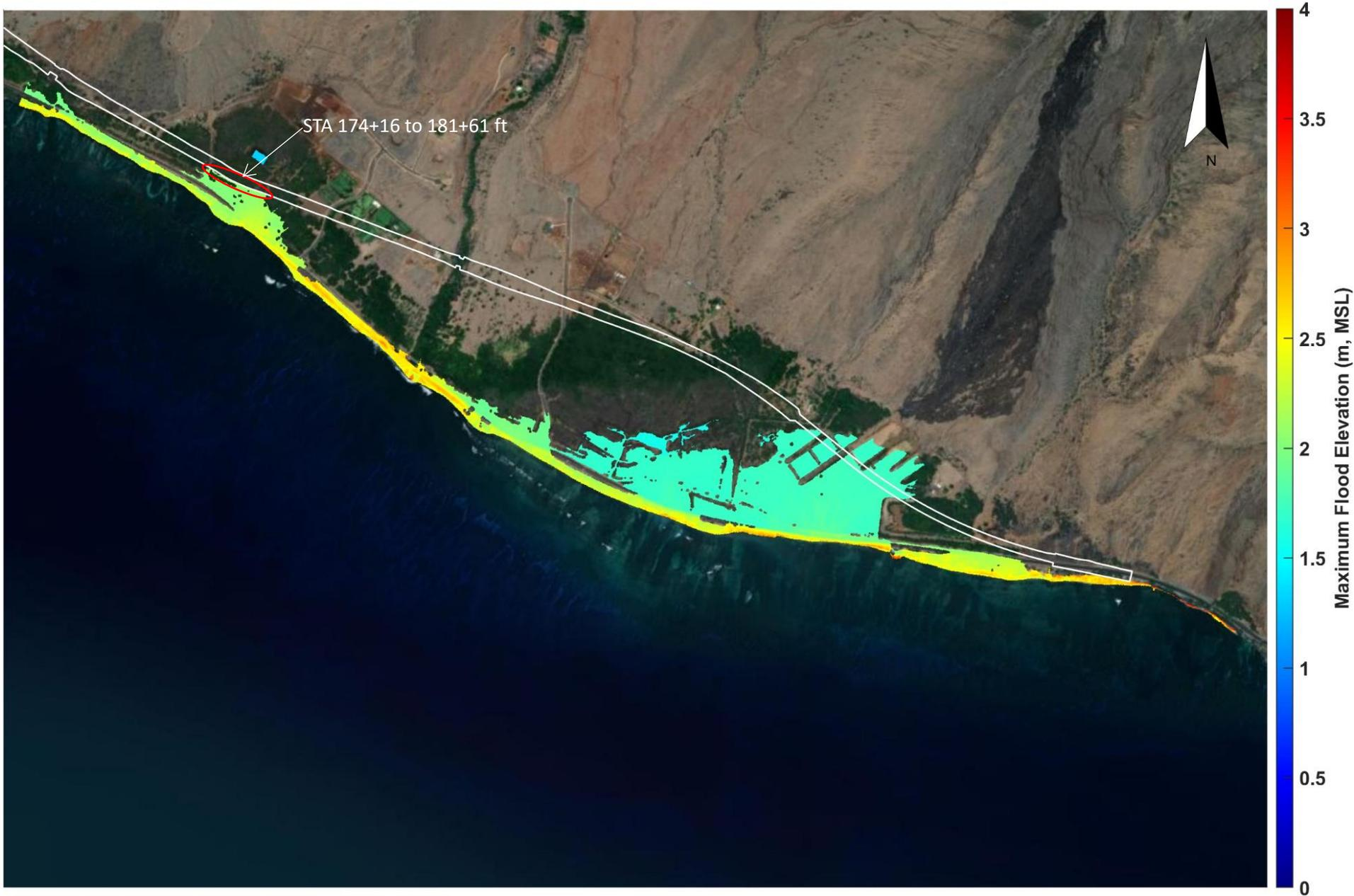
Figure F-2. XBeach-NH modeled maximum flood elevation for alternative 4 alignment (Ukumehame)
