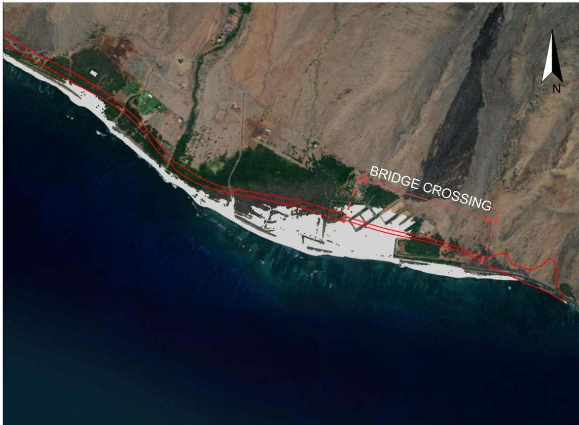
Figure 5-14. *Ukumehame* XBeach-NH modeled maximum flood extent (gray) for alternative 1 (red) alignment
