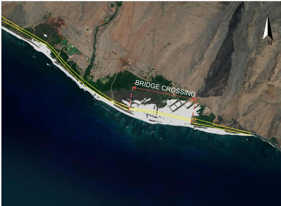
Figure 5-16. *Ukumehame* XBeach-NH modeled maximum flood extent (gray) for alternative 2 (yellow) alignment
