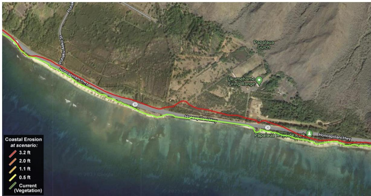
Figure 3-5. Erosion Hazard Model projection for shoreline location with 3.2 ft of slr at Ukumehame
