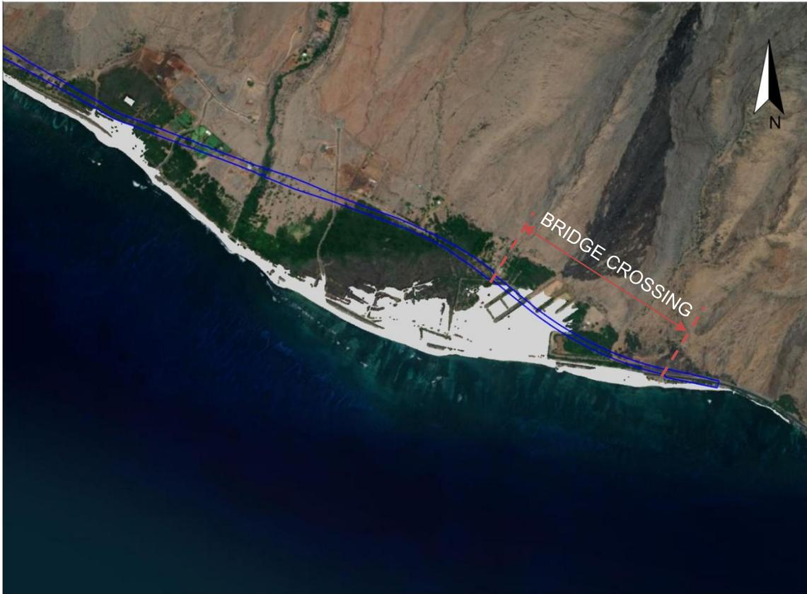
Figure 5-20. *Ukumehame* XBeach-NH modeled maximum flood extent (gray) for alternative 4 (blue) alignment
