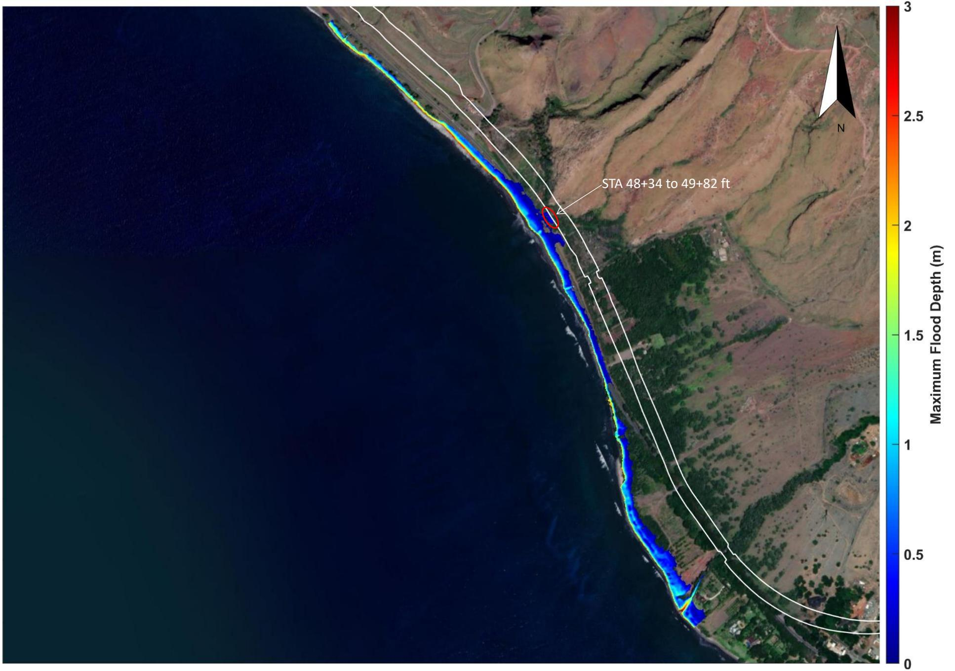
Figure C-4. XBeach-NH modeled maximum flood depth for alternative 1 alignment (Olowalu)
