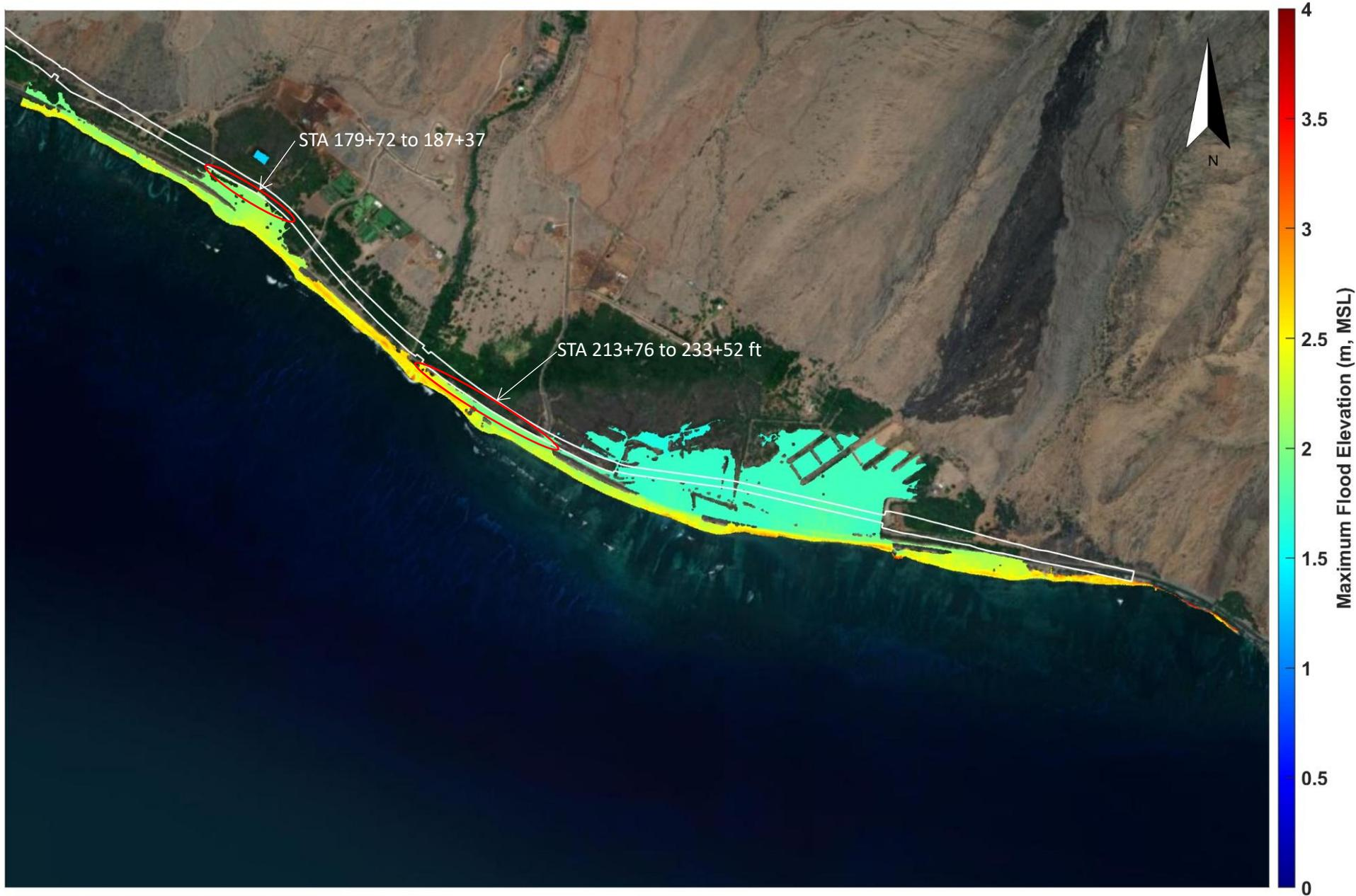
Figure D-2. XBeach-NH modeled maximum flood elevation for alternative 2 alignment (Ukumehame)
