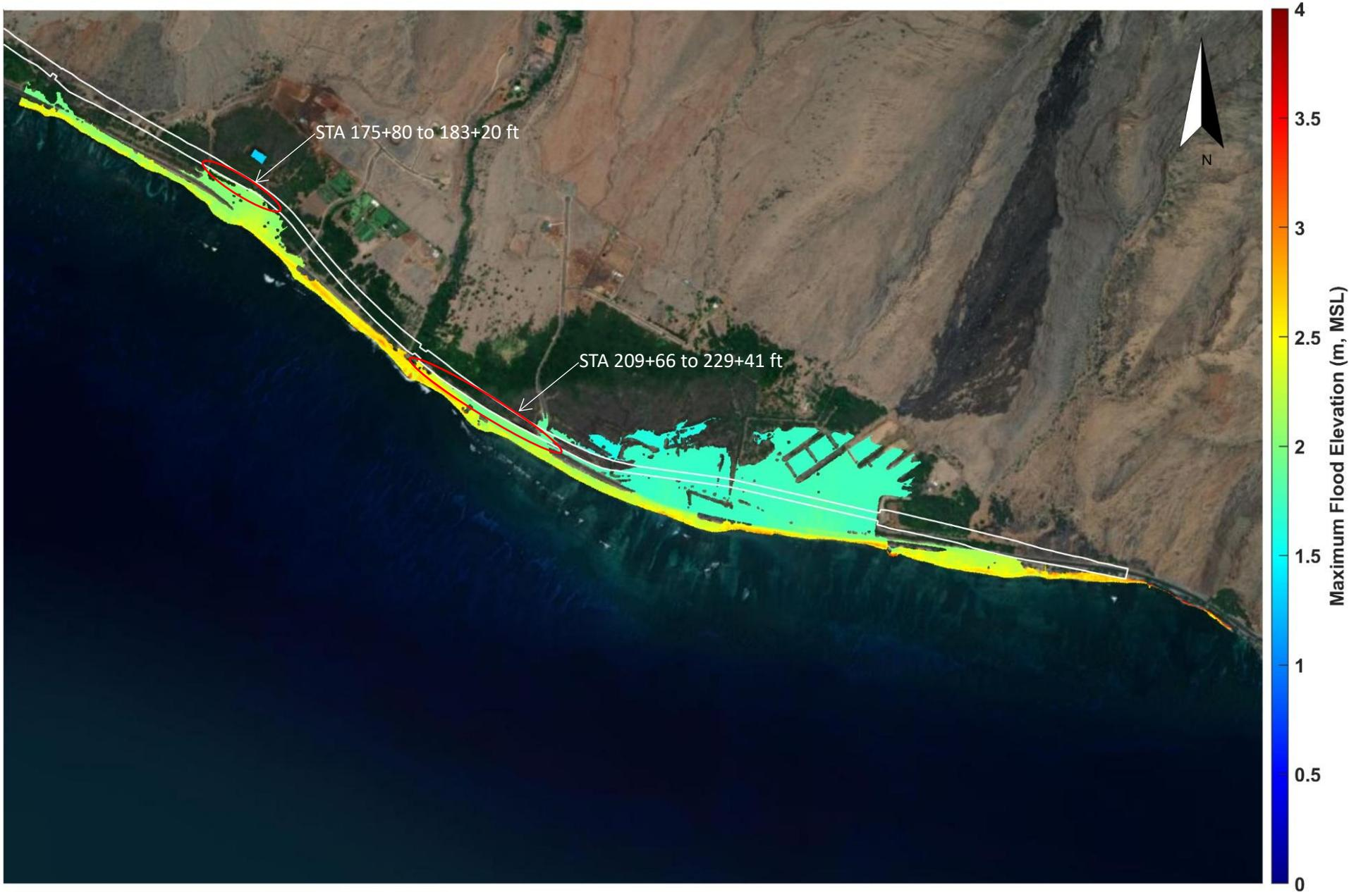
Figure E-2. XBeach-NH modeled maximum flood elevation for alternative 3 alignment (Ukumehame)
