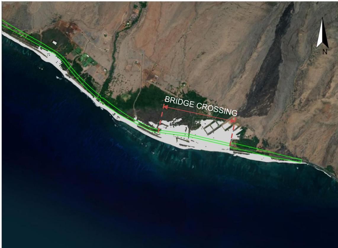
Figure 5-18. *Ukumehame* XBeach-NH modeled maximum flood extent (gray) for alternative 3 (green) alignment
