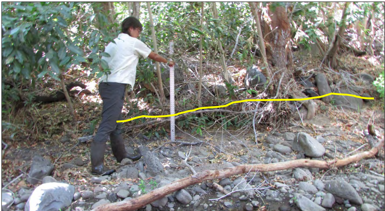
Photo 70. OHWM Level Indicators at Transect 1; OHWM Level Selected at the Elevation of Undercut Bank, Exposed Roots Below this Level, and Shelving of Debris Above the Level
