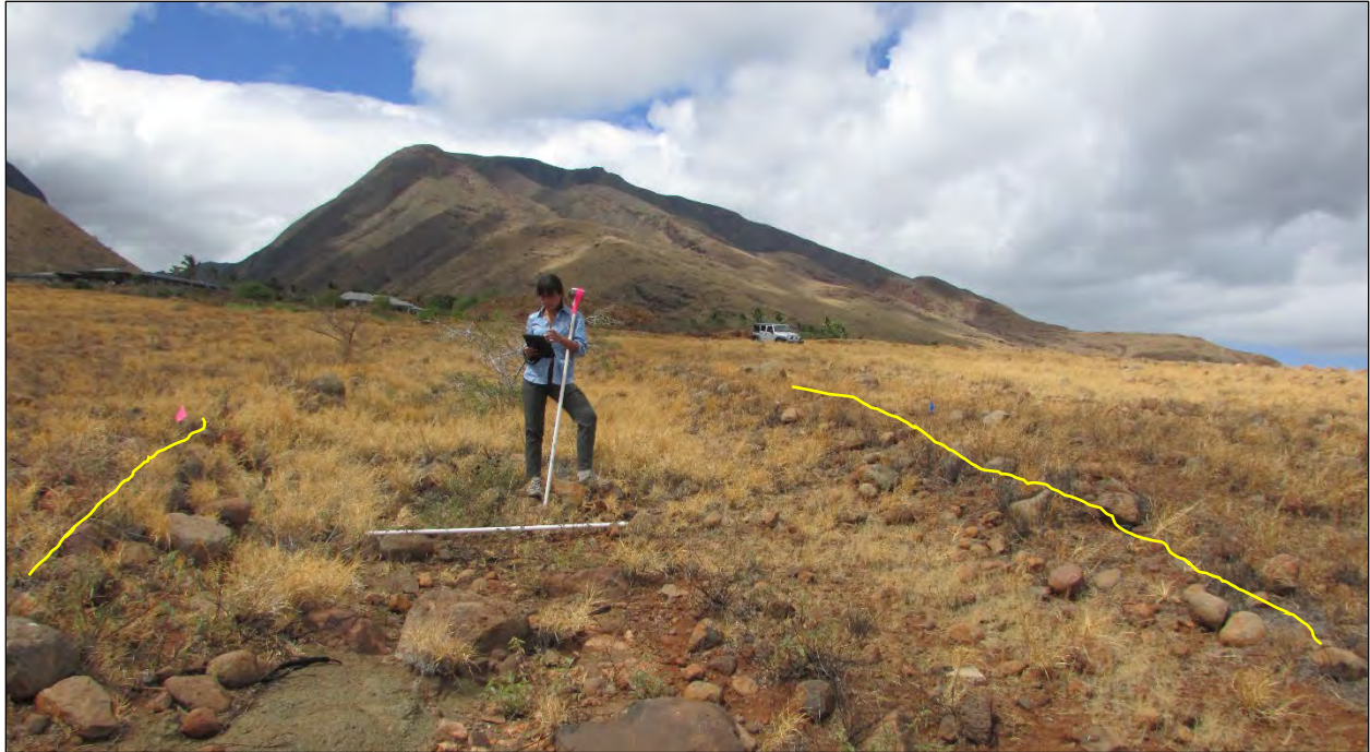
Photo 78. Mapua Stream – Shallow and Dry Stream Channel in September 2023; Break in Bank and Sediment Sorting from Boulders and Rocks to Sediment on Bank were Strong Indicators of OHWM in this System
